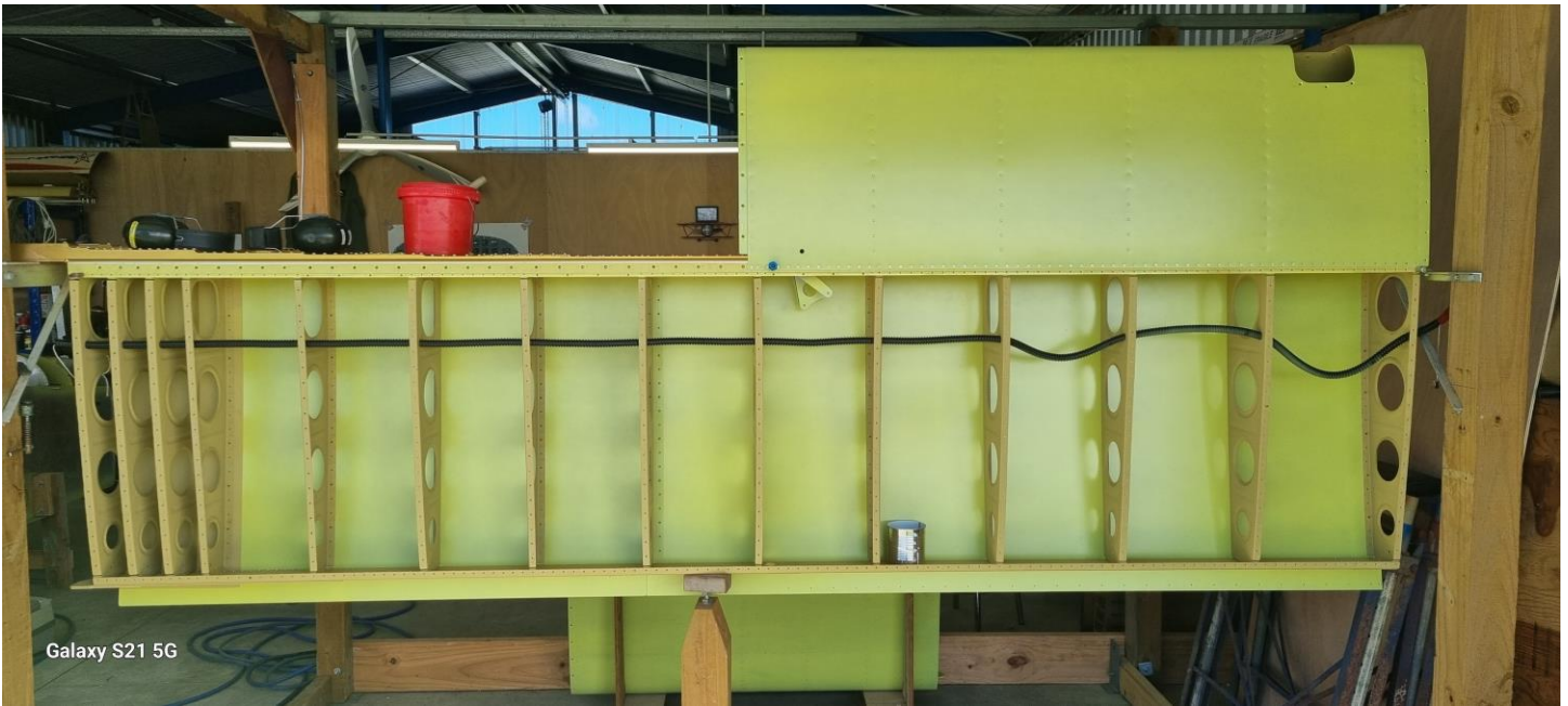
Above: LH Wing in Jig from underside, and tank not bolted (upper LH gap)
