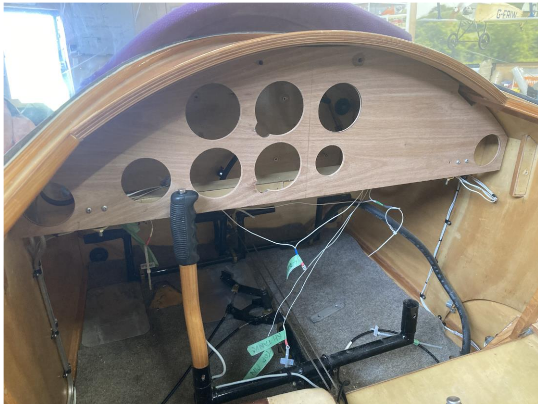
Below: Shows the new #5 panel in place, rubber mounted bottom and top.
