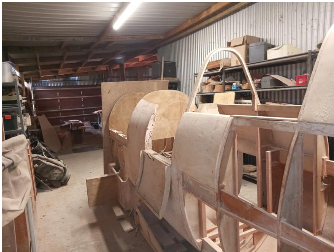
Above & Below: On the left hand side I have started to put the ply-sandwich panels in so I can get the entrydoor in place, likewise out of ply (6mm).
