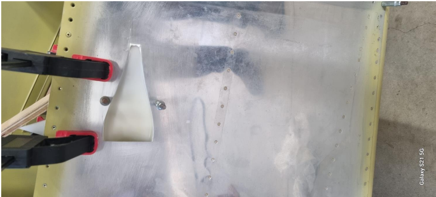
Above: Cold air intake with clecos in place and borrowed clamps (Ed: Hey! I recognise those)
