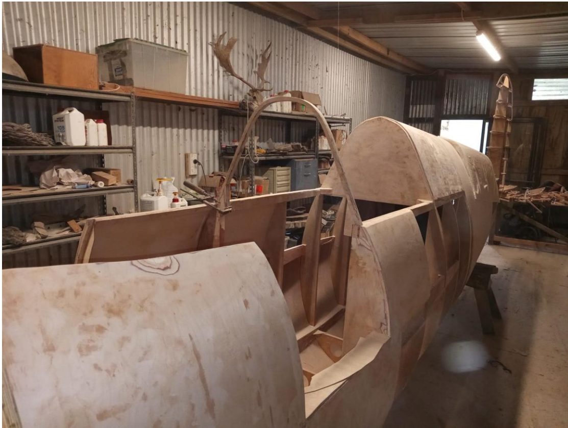
Above & Below: On the left hand side I have started to put the ply-sandwich panels in so I can get the entrydoor in place, likewise out of ply (6mm).
