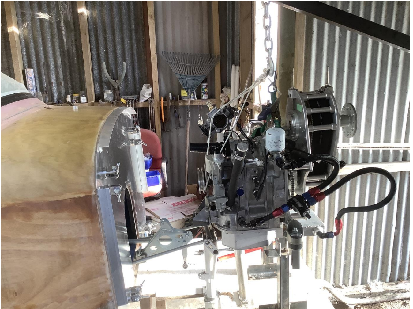
Above: Mazda 13b single rotor, Rotary engine with belt drive. It's loud, a bit thirsty but light and very powerful. It's shown here at Andrew's home base in Tauranga, but shortly to be moved to the Hangar at Matamata airfield for assembly.
