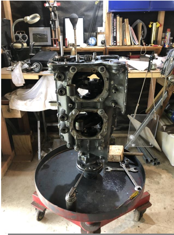
Above: Engine core stripped down and view in cockpit. Below: Instruments, very tidy against light birch panel, trim lever on right side.
