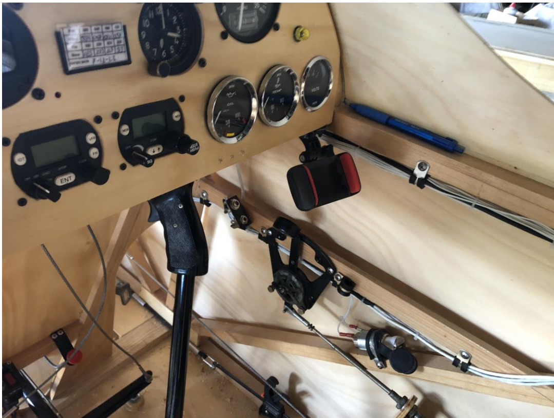
Above: Engine core stripped down and view in cockpit. Below: Instruments, very tidy against light birch panel, trim lever on right side.
