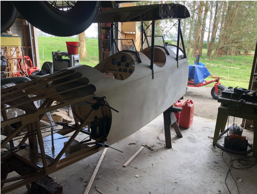
Above: Fuse on trestles with bracing being clamped Below: Throttle quadrant, very vintage look!
