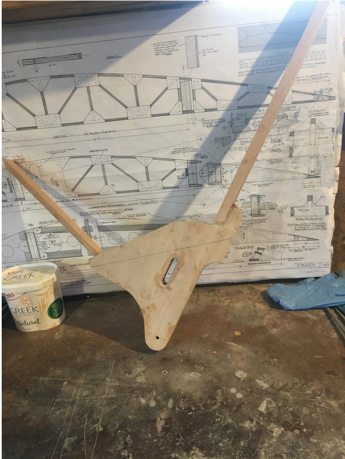
Finished Skeg ready for gluing into the Fuselage. Slot is for bungee for skid suspension which pivots on lower smaller hole. Pencil line is position on bottom of fuse.
