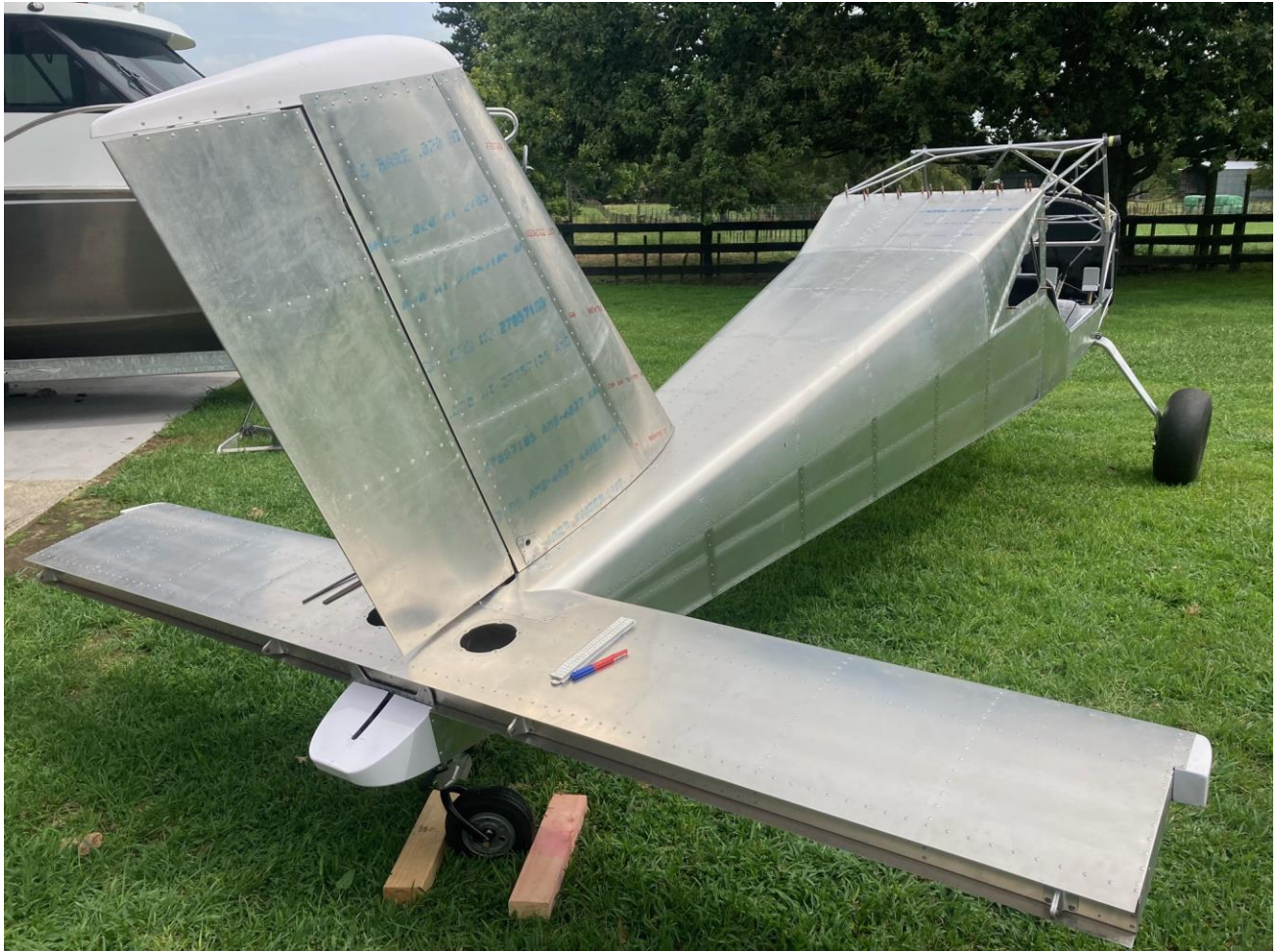
Picture above: view from the rear with stab fitted, no elevators in place yet.
