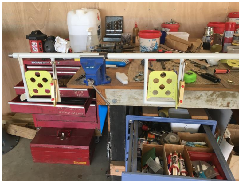
Above picture shows RV7a rudder pedals being assembled – upside down in vice...
