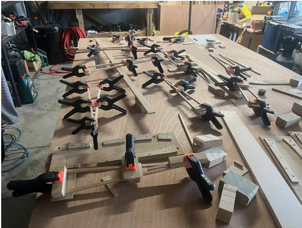
Picture above showing gluing of Corby Starlet ribs and some jigs...
