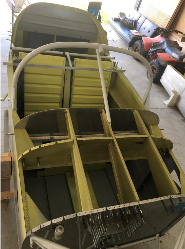
Above pic shows RV7a with front fuselage bracing and Canopy rollover protection in place.
