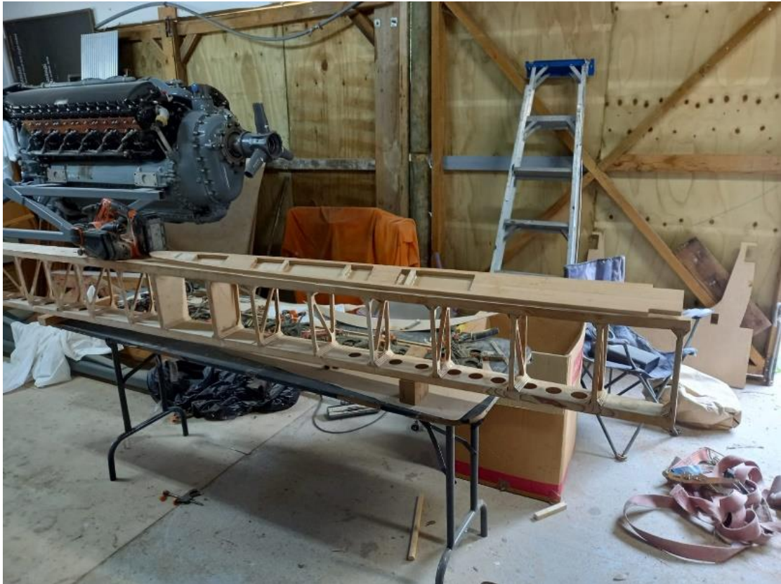
Above: Another view of dual tailplane spar truss which takes all the flight bending loads.
