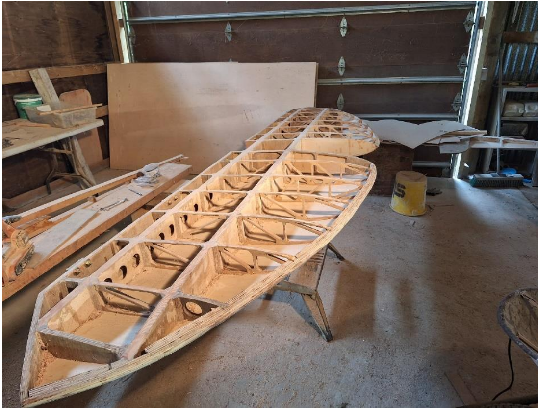
Above: bottom skin in place and leading edge shaped. LE is on RHS.
