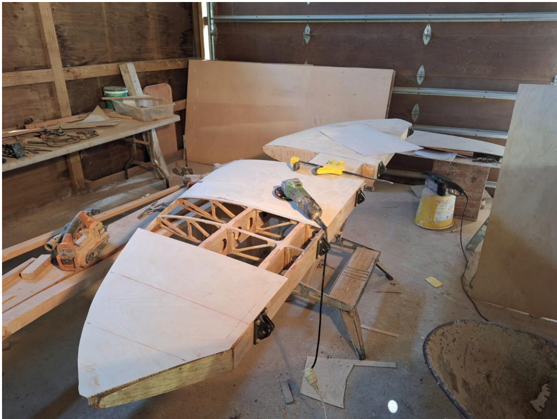
Above: Turned over with bottom skin and sanding and fitting skin. Hinges visible RHS, LE is LHS.
