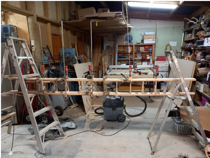
Above shows tailplane dual spar truss, initial construction, well clamped...
