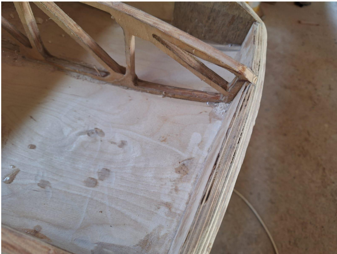
Above: Leading edge of tailplane showing bottom skin and laminating LE prior to shaping.
