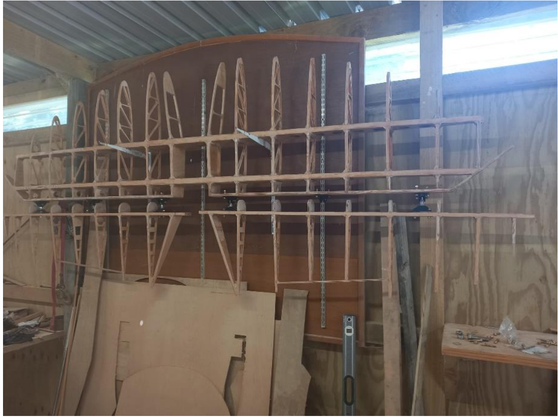
Above: View of whole tailplane with elevator attached (black hinges in middle)
