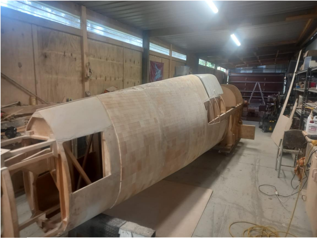
Above: Adding second skin of balsa to fuselage
