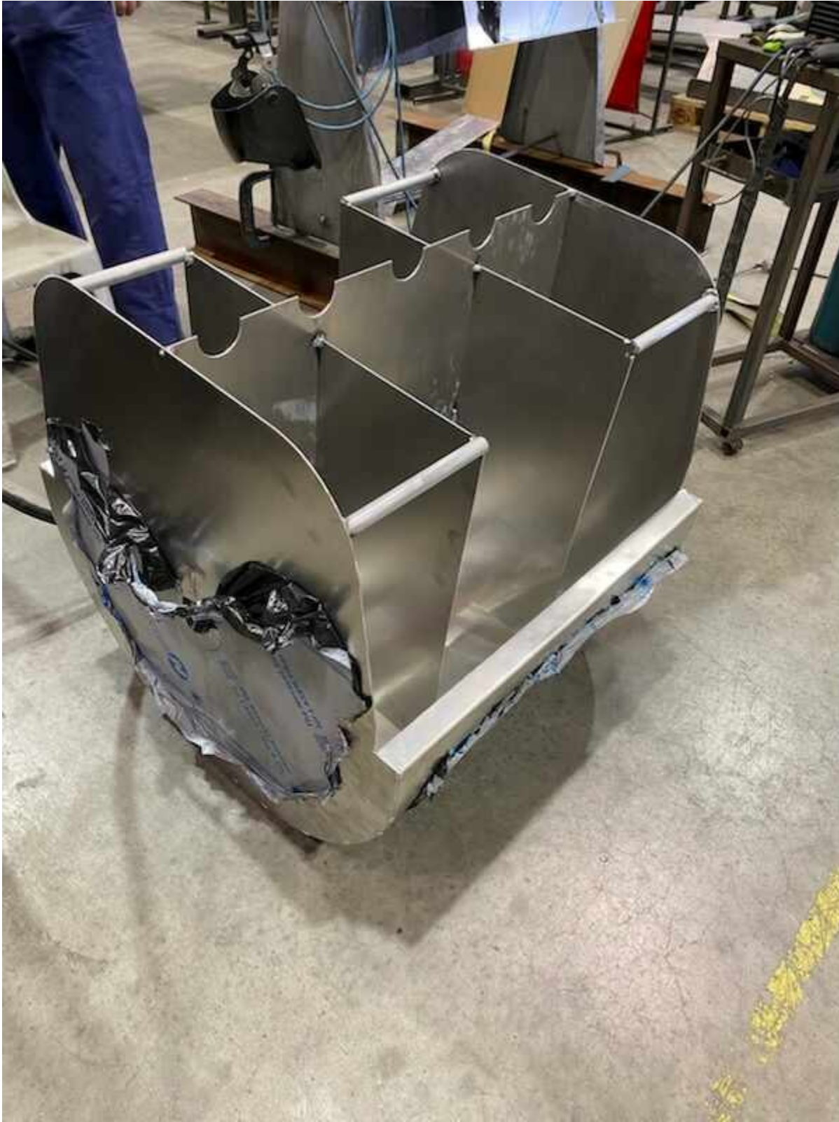
Below: Underside view of the tank, showing the internal baffles.
