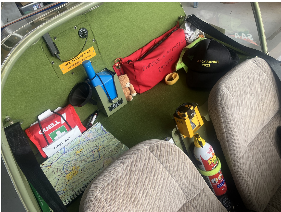
Below: Very tidy layout of parcel shelf, note USB/ADSB-in, PLB and fire extinguisher.
